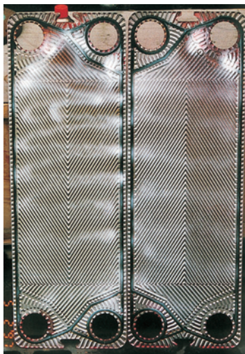
↑ Penetration cracking in red areas (the developing fluid by DPT)
