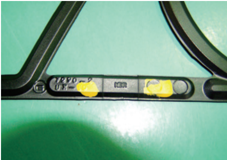
↑ With the lot number and yellow marking, it can be confirmed that this material is NBR.
