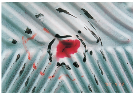
↑ Magnified of the fatigue crack
