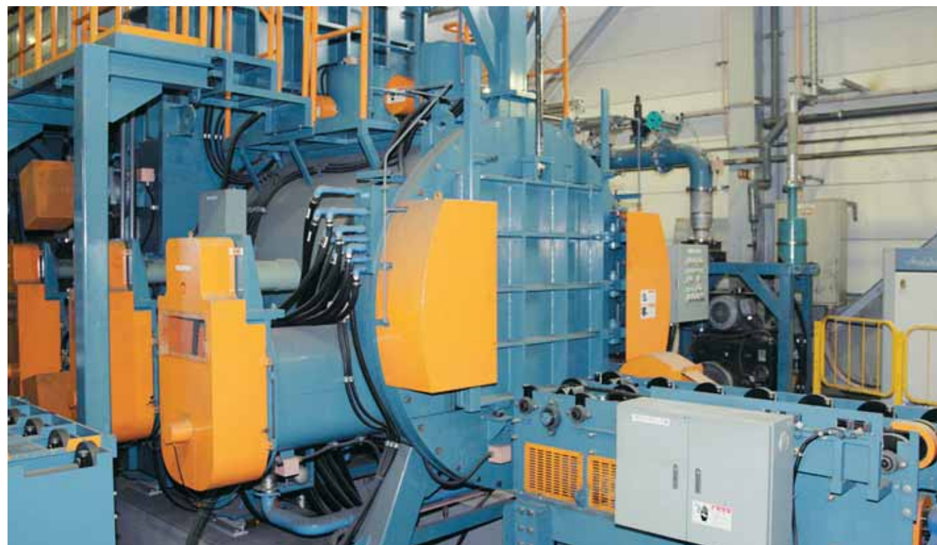
Continuous-vacuum heating furnace
