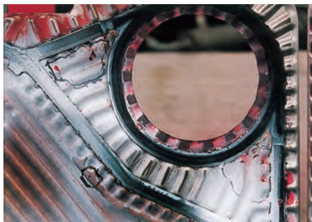
↑ Penetration cracking in red areas (the developing fluid by DPT)
