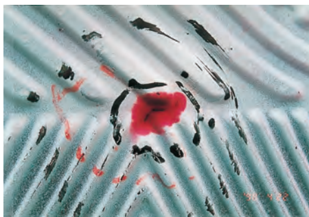
↑ Magnified of the fatigue crack
