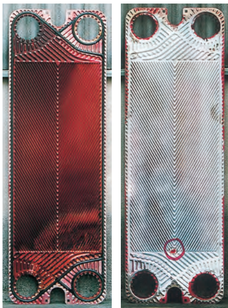
↑ Steam side (left) Thermo oil side (right)
