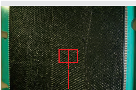
↑ Heat exchanger Seawater inlet port hole Wood chips, seaweeds and shellfish are blocking the flow channel, and causing poor flow in the unit.
