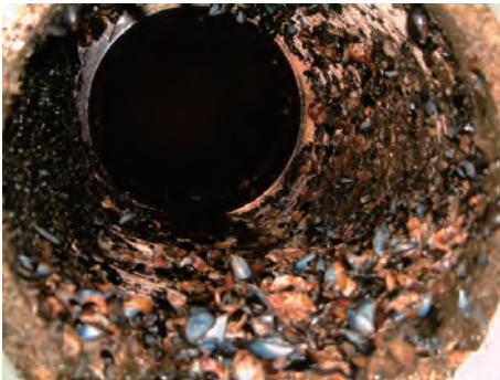
↑ Heat exchanger Seawater inlet port hole Wood chips, seaweeds and shellfish are blocking the flow channel, and causing poor flow in the unit.
