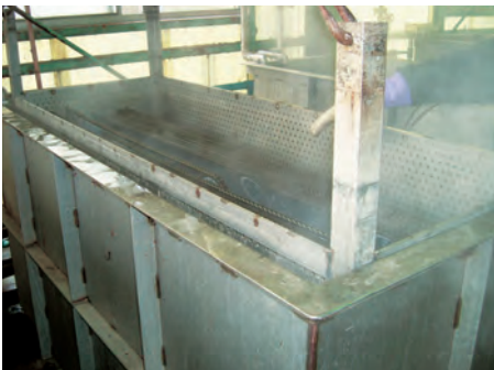
↑ Soaking in a chemical bath to remove hard scale.
