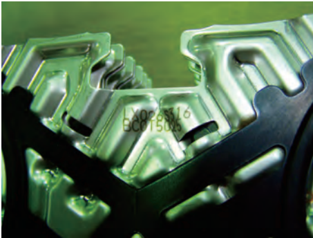
↑ Lot number Indicates that model LX-026, S316 is made of SUS316.
